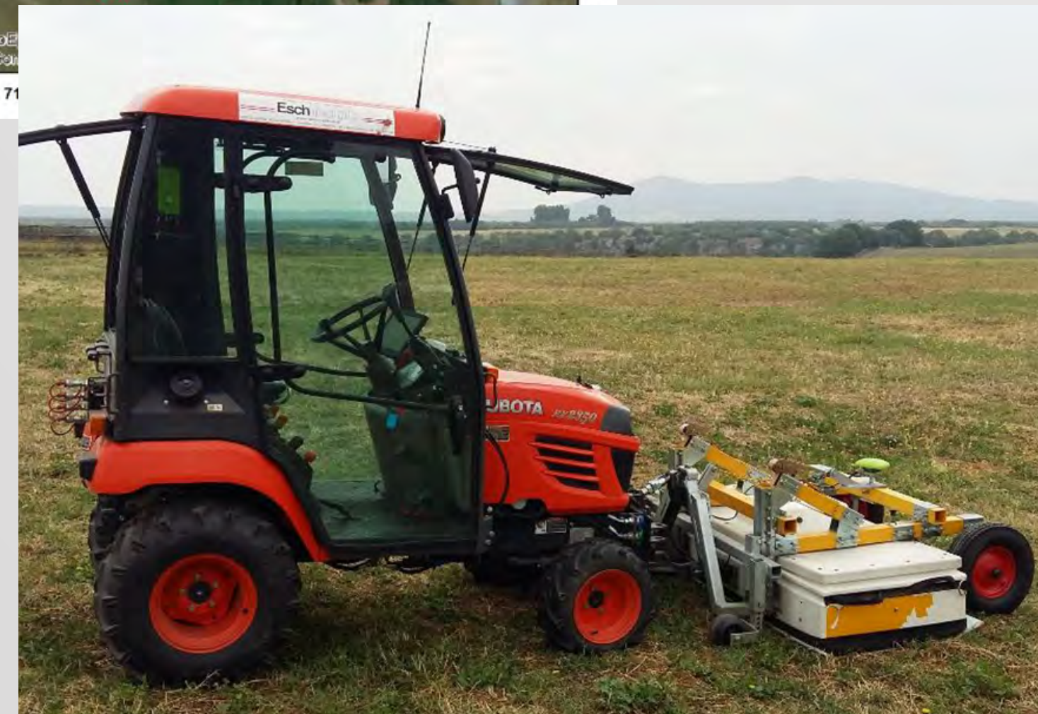
Pictured above is the 16-channel 400 MHz MALA Imaging Radar Array, onsite at Vulci, used to collect the new GPR data.
