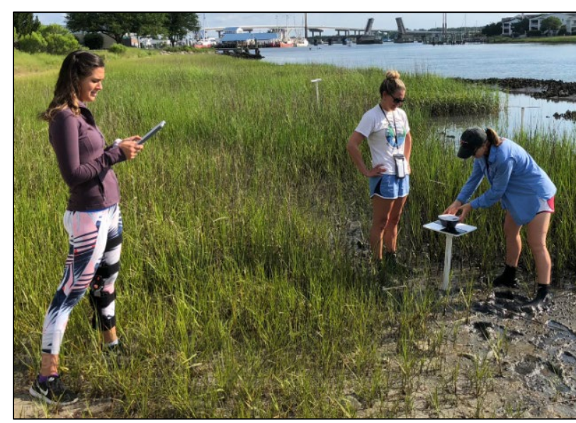
Above: Recording location of ground control points (GCPs) with a GPS, which improves data accuracy during processing.
