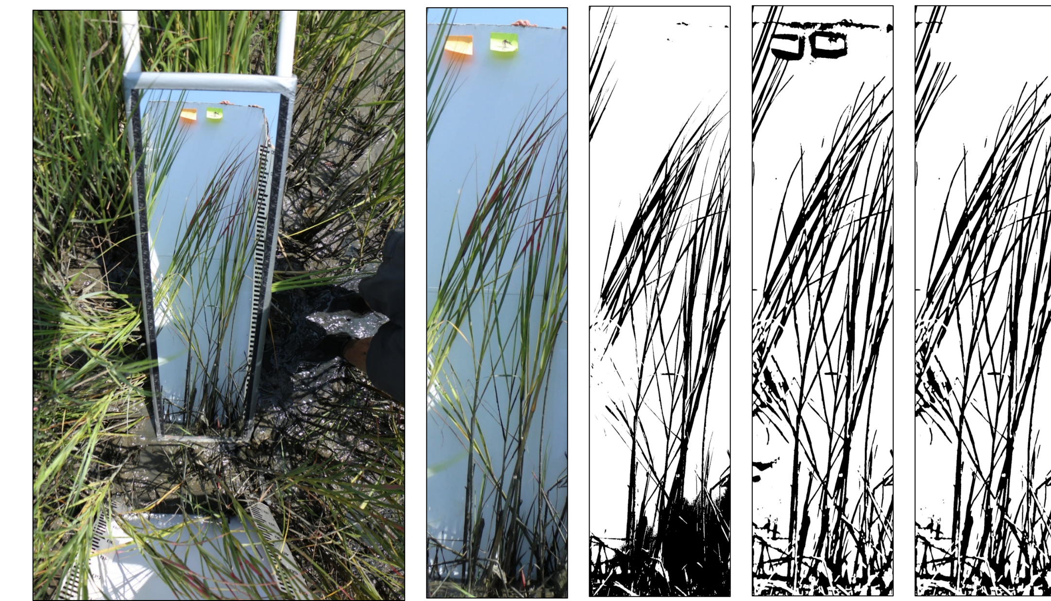
From left to right: Raw mirror image, Rotated and cropped mirror image, Global thresholded image, Adaptive thresholded image. Manually cleaned up adaptive threshold image ready for analysis.
