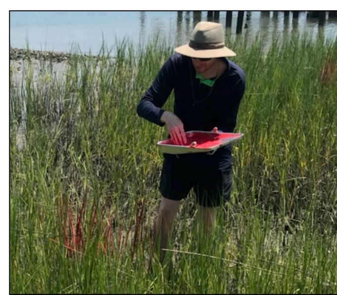
Above: Dr. Ridge uses non-toxic paint to cover marsh grass tops as part of the vertical accuracy assessment.
