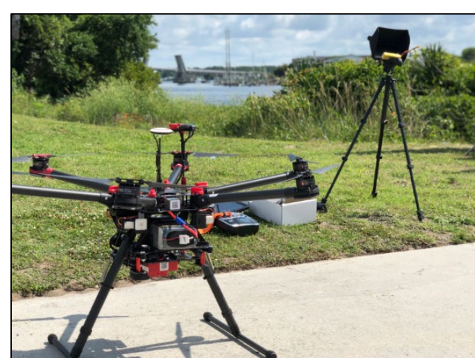
Above: Black Widow (DJI S900) drone used to collect project data.
