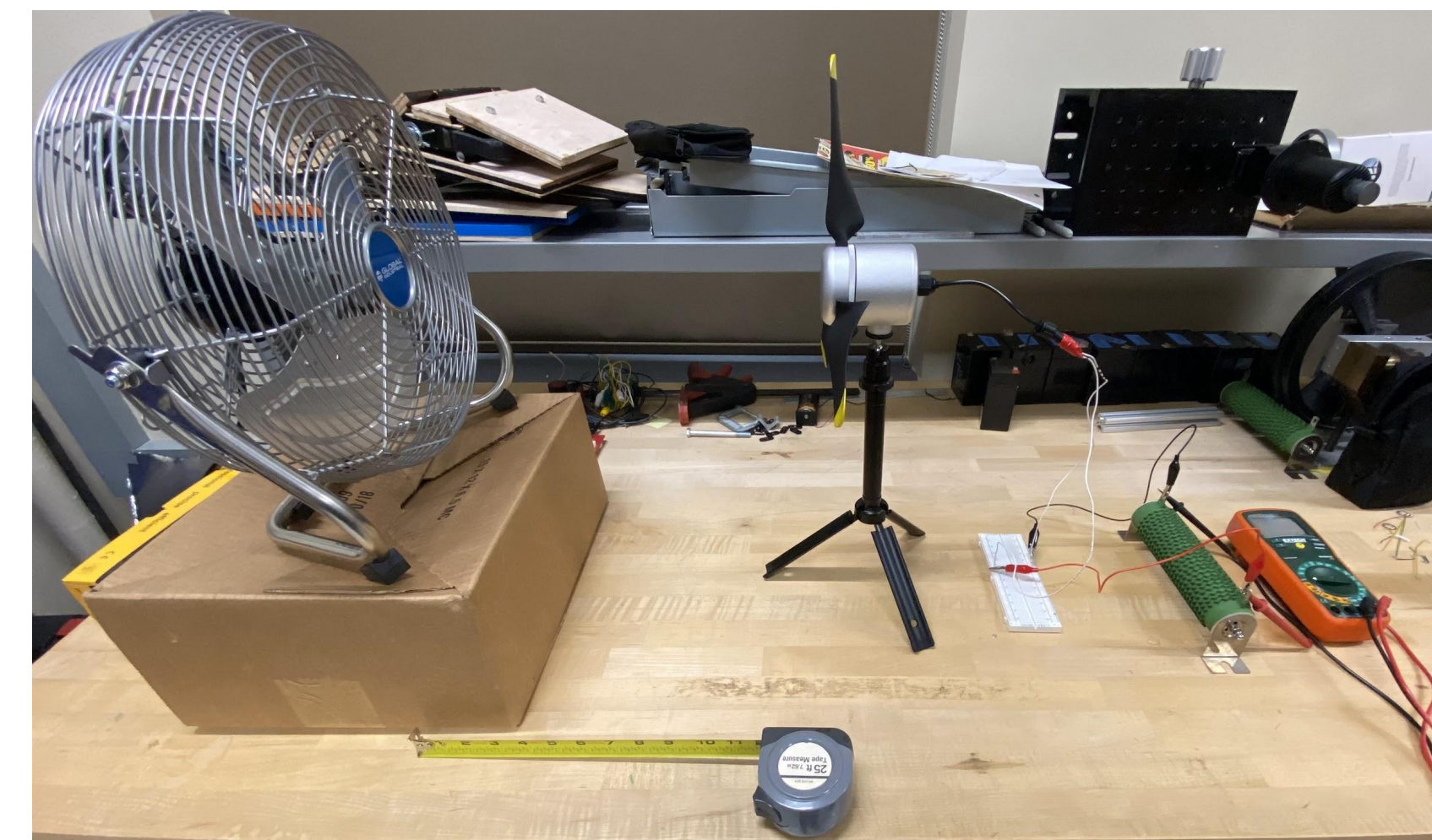
Figure 4. Test Setup Used for Both TexEnergy and Wind EnGen
