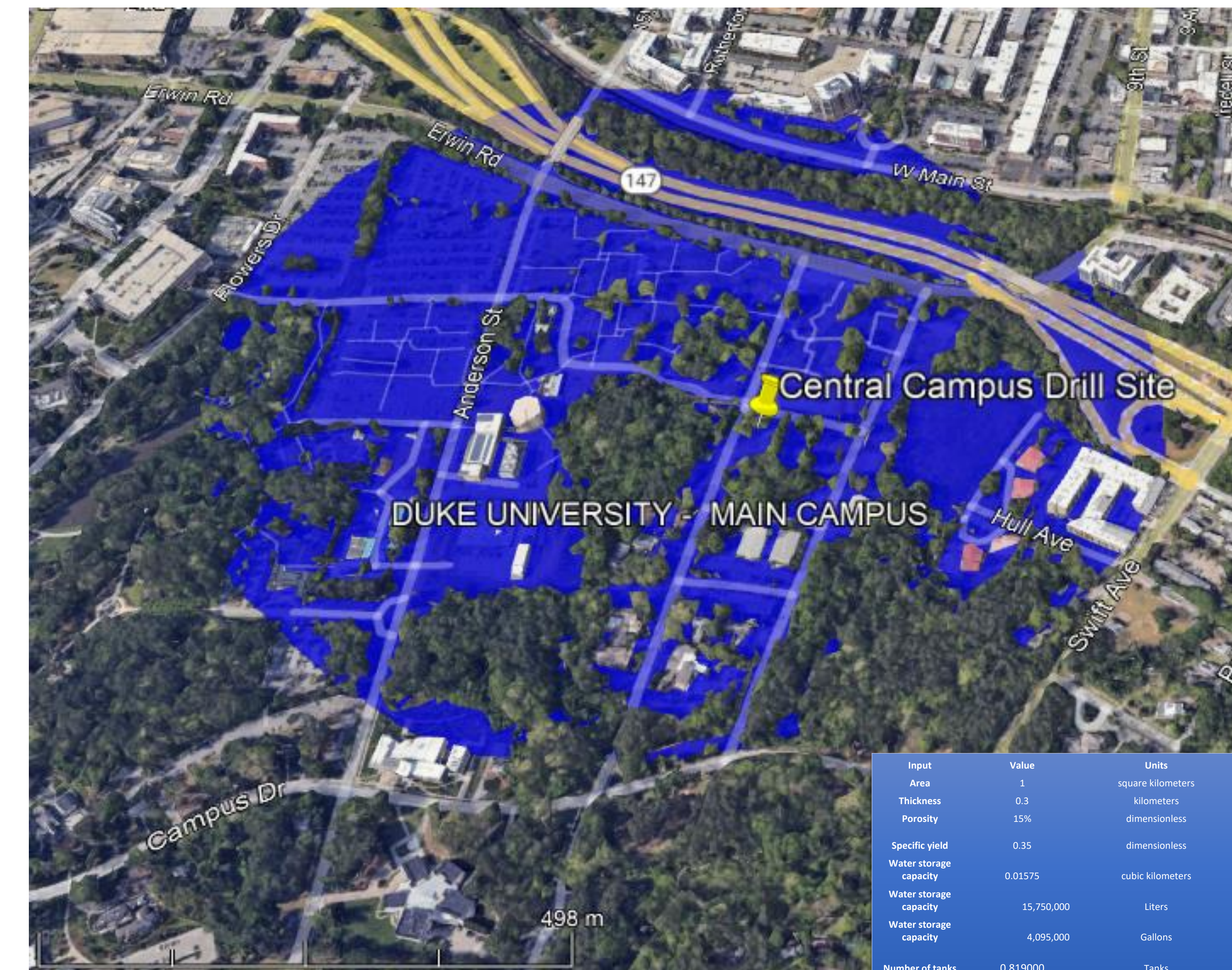
Figure 7. Proposed Water Storage Area for Aquifer Thermal Energy Storage System Near Duke University and Table with Estimated Water Storage Capacity 5 .
