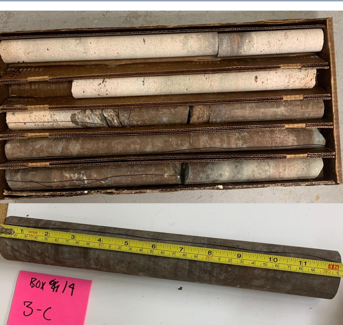
Figure 5. Soil Cores collected from Duke central campus well.
