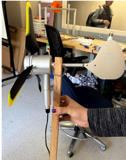
Figure 8: The wood block was put on the fin of the turbine to allow us to hold the turbine over the exhaust while standing at a distance
