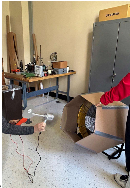
Figure 7: Testing the turbine setup with a nozzle and box fan
