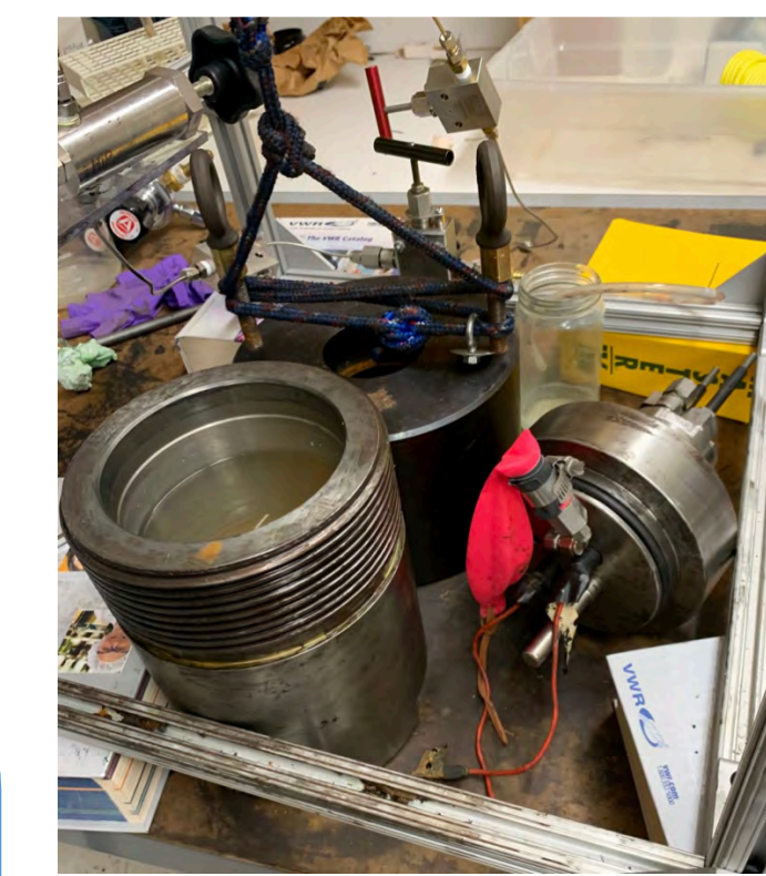
Interior of ultra-high pressure vessel with balloon attachment fitting
