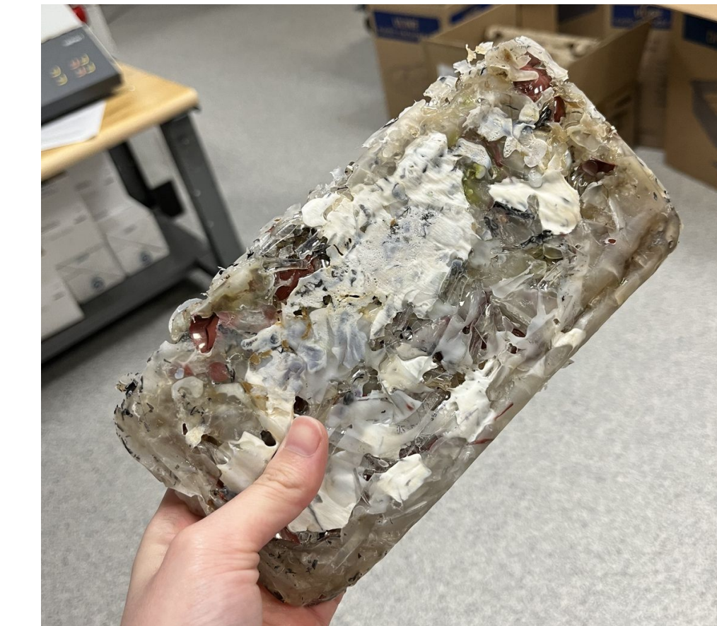
Picture 1. Completed Recycled Brick. Brick 4 containing 36% #1, 6% #2, 10% #4, 48% #5, total weight of 225.15g.
