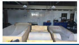
Above are the molds that will be used to create the carbon fiber body of the vehicle.
